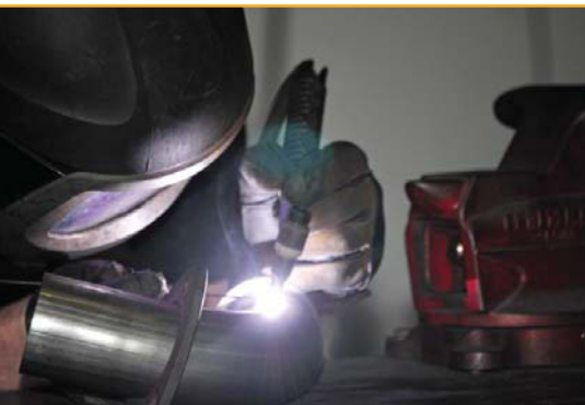
Chris Nixon welds a down pipe for a 1985 Land Cruiser with a diesel engine. TIG welding gives the technician the ability to get close to the pipe and make precision welds.
