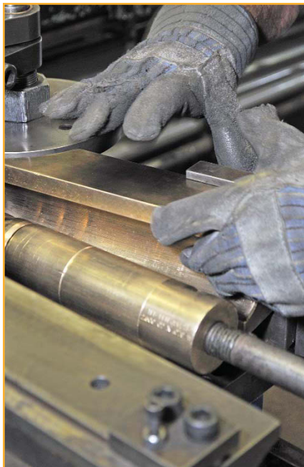
The mandrel bender is being prepared for stainless-steel pipe. Bronze dies are used for stainless steel, and chrome dies are used for aluminized steel.
