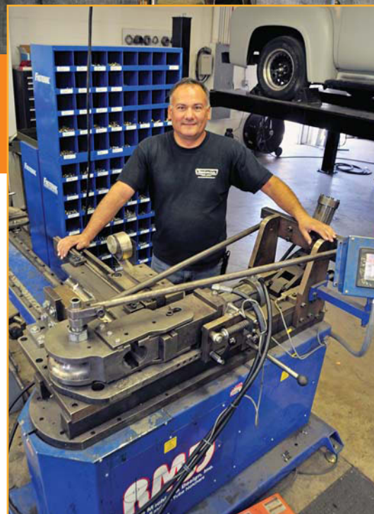
Henry "Hank" Padilla stands in front of his RMD MB-350 programmable, numerically controlled rotary-draw mandrel bender.
