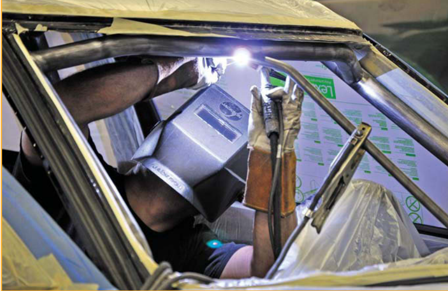
Hank puts finishing touches on a custom roll cage for a SAAB 900.
